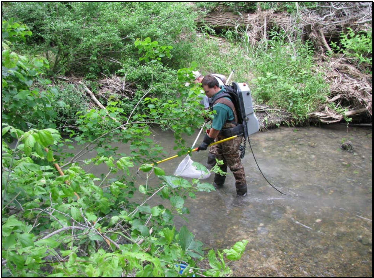
Figure 2.6. Sampling fish communities in Geronimo Creek using a backpack electrofisher at the Haberle Road sampling station.
